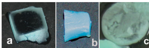
Figure 7 Photographs of chelated copper in gels; (a) cross-sectional view of copper chelated PAAm-AAm copolymer gel appears transparent inside and blue on the outside; (b) cross-sectional view of copper chelated PAAm gel appears uniformly blue inside and outside; and (c) cross section of the PAAm-AAm copolymer gel which turned blue outside and inside when placed in \text{CuSO}_4 solution. [Color figure can be viewed in the online issue, which is available at www.interscience.wiley.com .]
